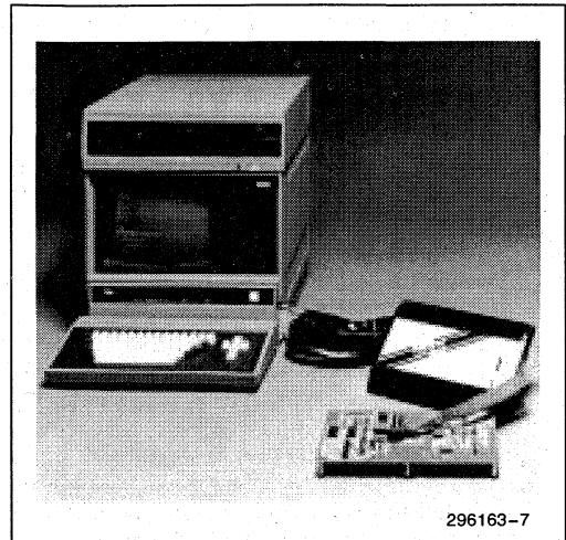
Figure 5. RUPI-44 Development Support Configuration Intellec System, ICE™-44 Buffer Box, and ICE-44 Module Plugged into a User Prototype Board
